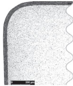
Micrograph of edge coverage with VACCOAT
